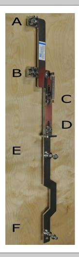
Fasten the line properly at "B". Twist the line through the guiding rails at "A".
